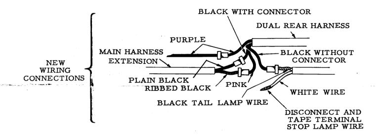
18. At the left rear side of the body disconnect the white colored stop lamp wire from the ribbed black wire and loop and tape the terminal.
