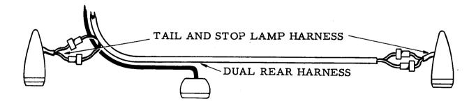
17. Connect tail and stop lamp harness to dual rear harness as shown.
