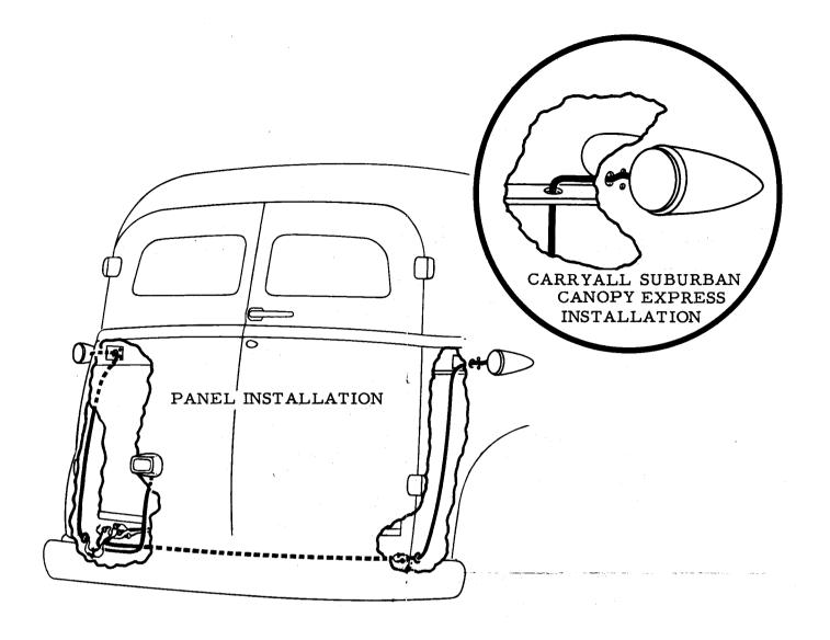
16. On panel models direct harness between insulating panel and outer panel downward. From underneath the truck, bring tail and stop lamp wires out thru hole in inner panel and insert grommet.
