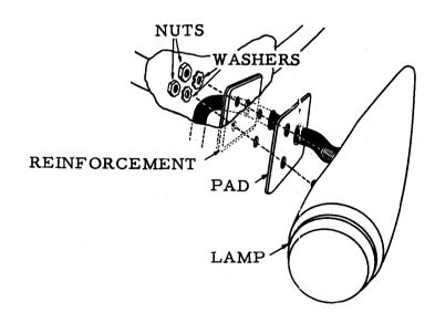
15. Mount lamp, pad, body reinforcement, washers and nuts in the order illustrated above.
